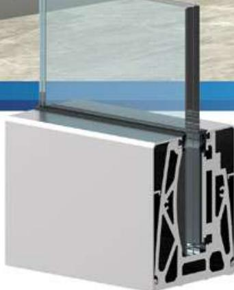
panorama XV10, the biggest benefit of using this system is the ability of aligning the glass panels upto  $\pm 2^\circ$  by fixing a set screw from the internal side. This ability helps a lot in projects where no handrail will be used on top of the glass. The system can be finished with one of the oval and straight cladding profiles upon your choice.
