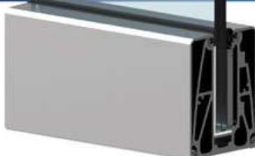
**panorama S10**, this system is designed to resist lower loads. You can use 5+5 mm or 6+6 mm glass panels at this system. The glass panels are fixed by the pressure plate which is activated by the set screws located at the internal side of the supporting shoe. You can choose one of our oval or straight cladding profiles to finish the system.
