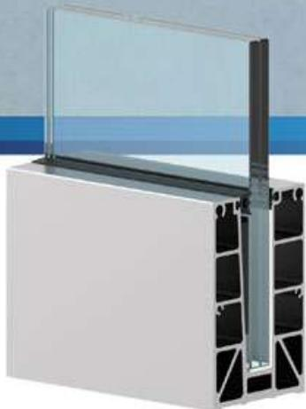
panorama M20-M21 systems are developed in two options. The one with oval form is called as M20 where the one with straight form is called as M21. These two systems are designed to be used as continuous rails. You can use 6+6 mm or 8+8 mm glass panels by changing the plastic spacers behind the glass. The glass panels are fixed with plastic wedges.
